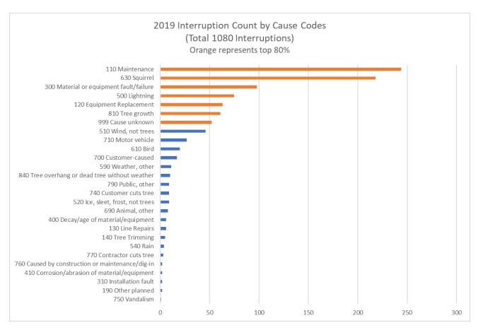
DKMT found, based on 2019 MillSoft OMS data, that about 40% of outages resulted from three maintenance and equipment related causes:
