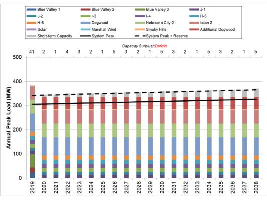
Figure 11-3: Power Supply Path 5 BLR
