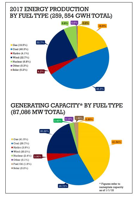
Figure 3-2: SPP Energy and Capacity Resource Mix
